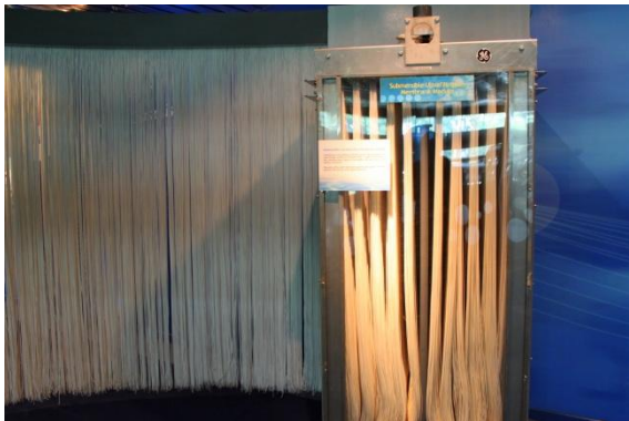
Figure 68 - The Microfiltration Membrane.
