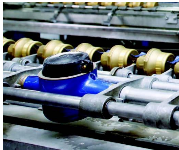
Figure 30 - Meters being tested on the indigenously designed hydraulic bench.
