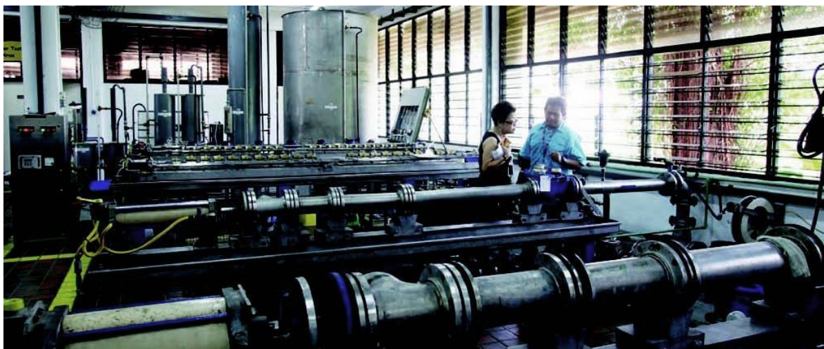
Figure 30 - Meters being tested on the indigenously designed hydraulic bench.
