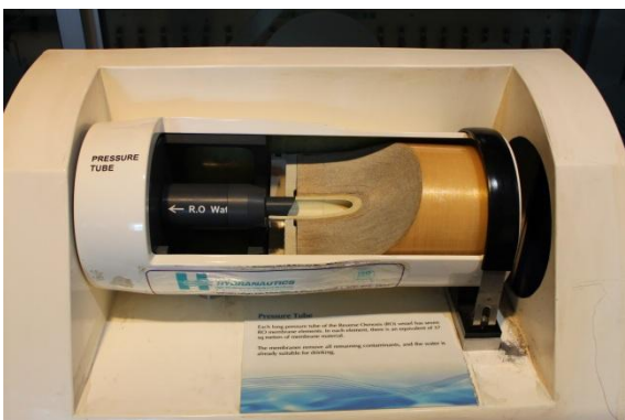
Figure 67 - The cut-section of the RO Module
