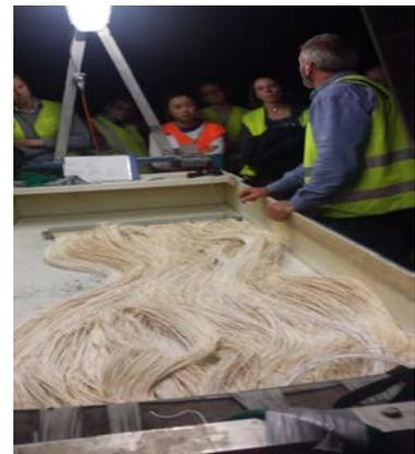
Zee weed have 500 membranes resembles the prefreated staw where the inside diameter of the viber is 0.8mm. As such the membrane can filter out more organic matters and therefore very less coagulant is added. This Zee weed system deployed about 6.5 million membranes fibres to create large surface areas and achieve 150 mega litres per day of flow through out the membrane pores.
