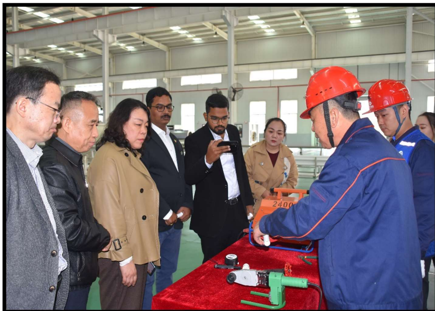
Demonstration of PPR pipe joining using electric fusion at Shaanxi Xingjilong Pipeline Co.Ltd
