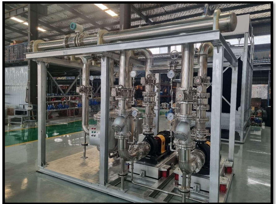
Prefabricated skid mount fire pump at Jin Lai Bang Valve Co.Ltd.
