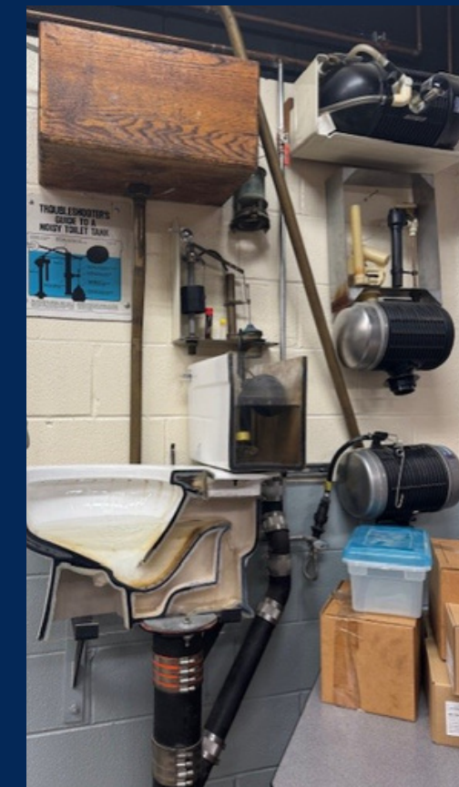
(Above - W/C rig for teaching and learning fault finding)
