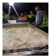
Zee weed have 500 membranes resembles the prefrated staw where the inside diameter of the viber is 0.8mm. As such the membrane can filter out more organic matters and therefore very less coagulant is added. This Zee weed system deployed about 6.5 million membranes fibres to create large surface areas and achieve 150 mega litres per day of flow through out the membrane pores.
