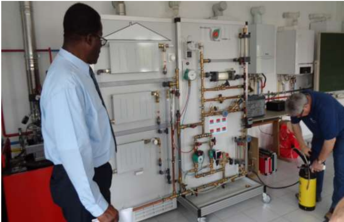
Picture 4: Master at Schienfurt Guild of plumbing charging up heating simulator to measure pressure drop through piping components
