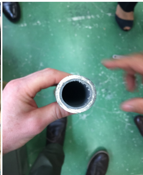
Figure 90 (Galvanised steel with inner plastic lining)
