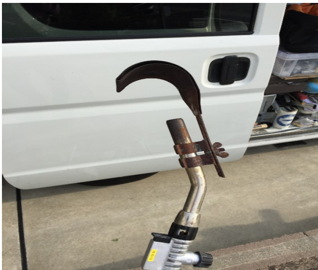
Figure 75 (To prevent the wall burning when soldering)
