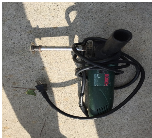
Figure 76 (To cut soil or waste pipe internally)
